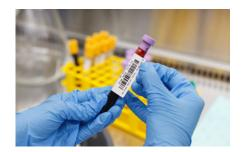
On top of this, the B-492 'FreezerBondz' label that could now be printed almost automatically, isn't just any label. It perfectly fits tubes, it can resist common laboratory chemicals and the label stays legible and attached in liquid nitrogen storage temperatures at -196°C, when printed with the BradyPrinter i3300.
