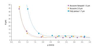
Accucore Vanguish UHPLC columns are more efficient at optimum flow than sub-2 μm fully porous and 2.6 μm solid core columns. Efficiency is maintained over a wider linear velocity range.
