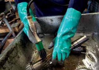
The mechanical strength of chemical gloves are determined through testing to EN ISO 388:2016 which covers abrasion, cut, tear and puncture
