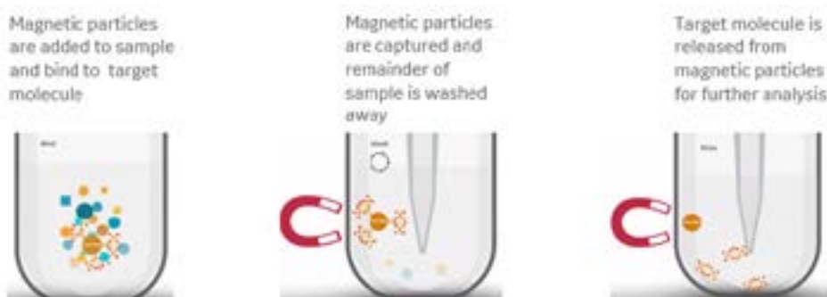
Fig 4: Overview of magnetic bead-based nucleic acid isolation. (A) Target nucleic acid in the sample binds to beads based on buffer conditions. (B) Magnetic field immobilizes magnetic beads while unwanted debris and contaminants are washed away. (C) Beads release target nucleic acid by changing buffer conditions.
